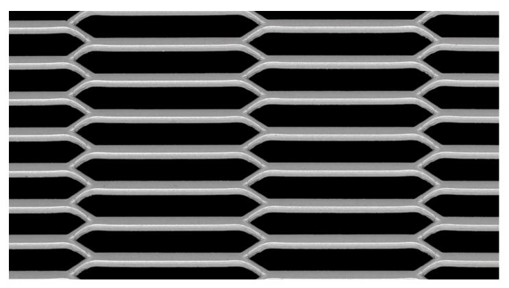
3.00mm LW Pitch: 133.33mm Strand Width: SW Pitch: 12.90mm Thickness: 3.00mm Weight: 10.50 kg / m2 (Black Weight) Open Area: 53%
